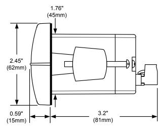
Figure 5. Meter Dimensions – Side View
