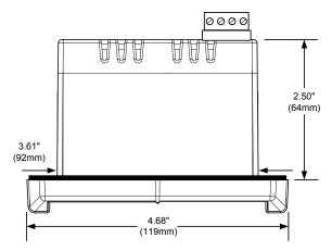
Figure 6. Case Dimensions – Top View
