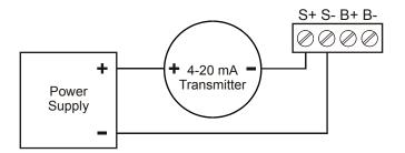
Figure 4. Input Connections without Backlight
